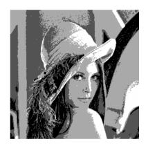
[Artifact] quantization error [Solution] increase number of quantization levels
